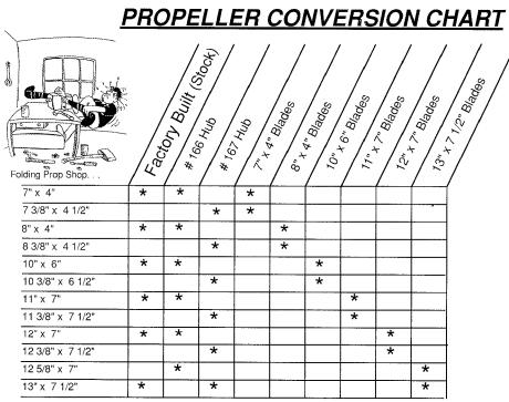
**Propeller "Pitch & Diameters" available by interchanging Blade and Hub assemblies.** NOTE. . Our 6" x 4" propeller parts are "not" interchangeable !
